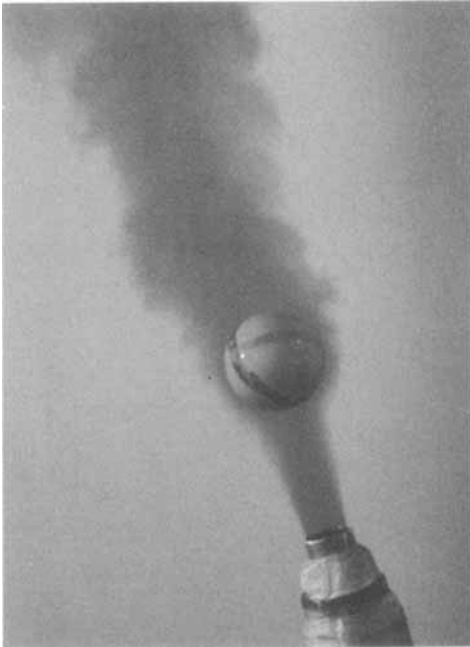
FIGURE 11. Flow around a sphere in an inclined jet. (a) Normal rotation of a ceramic sphere. \rho = 3.813 , G = 1.227 \times 10^7 , \alpha = 12.5^\circ , \kappa = 2.236 , Re = 9.838 \times 10^4 , (x/D, y/D) = (4.354, 0.8422) and \Omega = 0.03857 . (b) Anomalous rotation of a rubber sphere. \rho = 1.185 , G = 1.608 \times 10^8 , \alpha = 10^\circ , \kappa = 1 , Re = 1.652 \times 10^4 , (x/D, y/D) = (3.174, 0.4387) and \Omega = -0.2325 . One may note that the jet is deflected to the left (a) or the right (b) depending on the direction of rotation.
